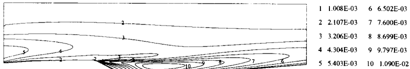
Figure 12. Turbulent kinetic energy pattern for flow over sand dune
